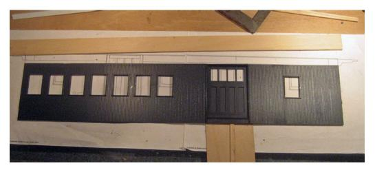
Glue on the sill - be careful to make it upright, at right angles to the sides (this is tricky, as there is nothing to hold it at the right angle. You could put a thin piece of scrap along the inside top of the scribed side piece to give you a wider gluing surface.) Again, clamps and scrap will help keep it in place while it dries. When you pick the side up, run your glue along the joint(s) behind the side to strengthen it. Test it again on the underframe, and file to fit if necessary.
