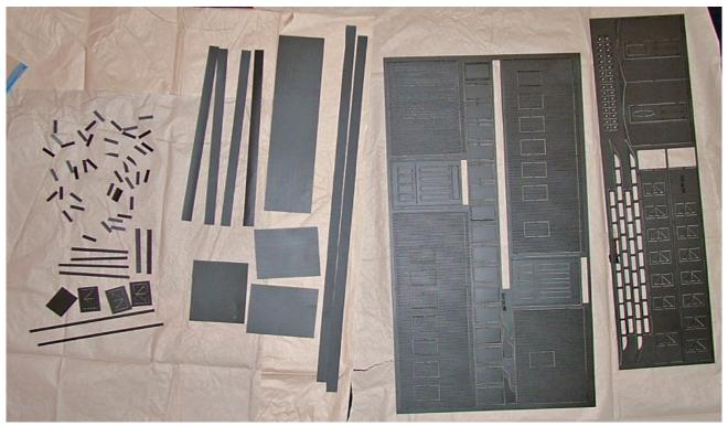
Take the kit and remove the parts from the styrene sheets. I use a chisel blade in an Exacto #5, but a knife will work. Sand and file off the tabs where the parts were attached. In particular, do a neat job on the window surrounds as they are pretty visible when you're done. (There's a spare in case you break one.)
