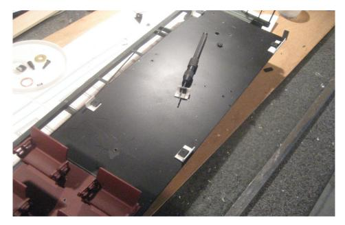
Once the tabs are glued and you are satisfied with the fit, you should carefully unscrew the sides from the floor and see if you can lift the body off around the seats. It can be a tricky fit. If not, re-arrange your seats; moving the tabs is a lot more difficult (but not impossible - just re-drill the holes in the metal floor, but make sure you clear the plastic underframe.)
