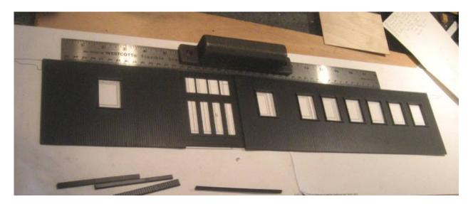
The door is flush with the top of the sides. Arrange the sides and the door on top of your template (that you checked against the original sides when you took them off - right?) Put a straight edge along the top line, and support the ends of the sides with some scrap styrene - the rectangles you popped out of the window work - so they rest on the door sides and all is flat and square. Glue the sides to the door, checking the length again before the glue dries.
