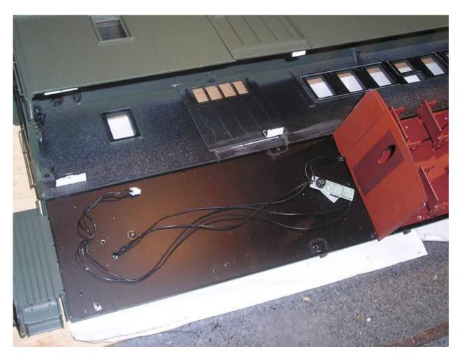
Note: you probably noticed when you unpacked the coach that the wheels don't rotate very easily. The main problem is the wheel wipers picking up power for the lights. A much better solution (my opinion) is to remove the wipers and fit a 9v battery and on/off switch or similar in the coach. I used a standard non-rechargeable type, as I don't use lights very often. If you do, I'd suggest a 4 x AA pack with a recharge socket under the floor in the baggage area.
