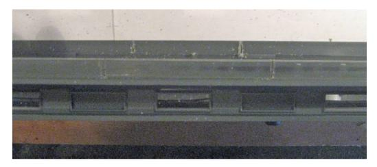
Cut the letterboard down to the roof but no more with a small saw. Make it slightly smaller than marked - you can always widen it but it won't be easy to make it narrower. I snapped out the strip by scoring along the edge of the roof with a sharp knife, and then I gripped the end in pliers and carefully bent it until it started to break. Repeat at the other end and the strip will pop out. File the rough bits down and check the fit.
